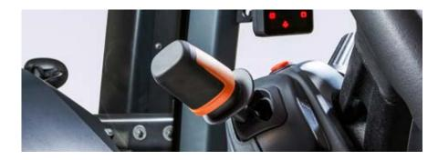
Integrated park brake / The fully integrated and easy to use park brake, reduces stress and unnecessary hand movements during loader work. Placed perfectly behind the steering wheel, it is easy to reach.
